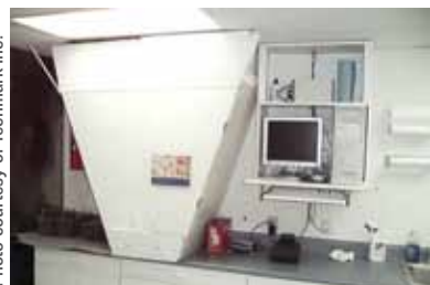
Techmark Approved Labs use lightboxes to take consistent photos of processed potatoes for quality evaluation.
