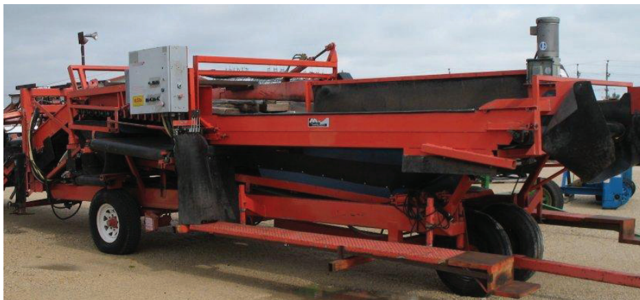
60" Milestone Star Table Dirt Eliminator with Hyd Adjust Stars, 2 Belted Stingers, Excellent Condition
