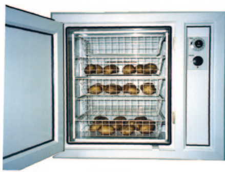
The Potato Hot Box speeds up the reaction time of potato tubers to show physical effects of bruising.
