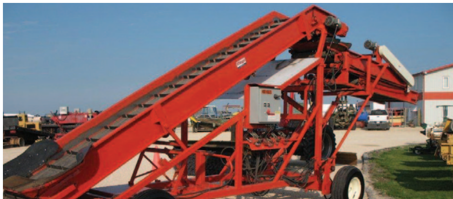
30" wide Mayo Telescopic Planter Filler with 180 Degree Swinging Boom, Deep Cleated Belt, Hydraulic Ground Drive & Steering, Very Nice
