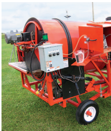
The Milestone liquid seed treater is the preferred technology for applying Cruiser Maxx D Potato.
